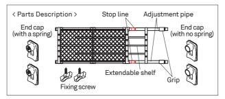
2) Rotate the grips in the direction of 【つっぱり】 "stretch (press against wall)" to check that the grip operates properly. Then rotate the grips in the direction of [ゆるむ] "retract (loosen)" until the grip end returns approximately to the start line. Excessive retraction may cause mechanical damage.
