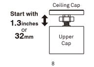
Measure the ceiling height. Cut the 2x4 lumber(\*) to a height that is 3.8 inches (95 mm) shorter than the ceiling height. \*Use commercially available 2x4 lumber (1 ½ x 3
