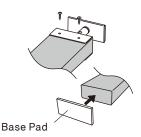
•Install the adjuster at the top and the base pad at the bottom of the pillar. Failure to do so could result in the product falling down.
